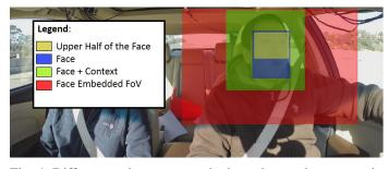
Fig. 4: Different region crops on the input image that are used to train the CNNs. The crop regions are color coded for clarity.
