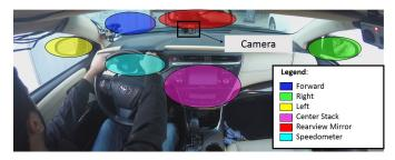
Fig. 2: Illustration of the driver gaze zones considered in this study. We also highlight the approximate locations of the camera used to capture the input images.
