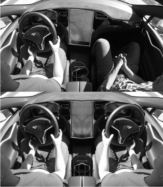
Figure 3: The symmetry-mirror augmentation used to reduce annotation time. (Top) Original camera image with both driver and passenger. (Bottom) Augmented camera image with driver mirrored to passenger side.
