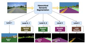
Fig. 3. The proposed hierarchical semantic structure. Support area includes sidewalk, ground, terrain, curb, and drivable areas; vertical area includes person, car, building, wall, bridge, tunnel, fence, vegetables and road utility; drivable area includes road, parking, crosswalk, lane marking, bike lane, service lane, catch basin, manhole and pothole; lane marking area includes dividing/guiding/turning markings, and stop lines.
