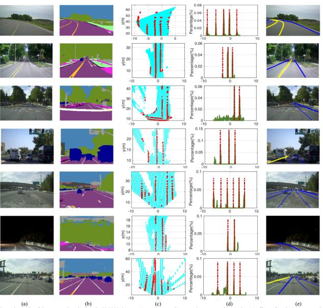
Fig. 8. Example results of the proposed method on the X-3000 dataset, (a) raw images, (b) semantic segmentation results, (c) offsets after slope compensation (red for lane points, cyan for road points), (d) histograms (green lines) of lane offsets and the detected peaks (red dashed lines), and (e) lane detection results, where blue/yellow stands for white/yellow lane line, line styles are also marked through solid/dashed lines.
