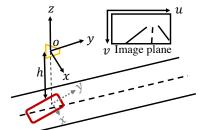
Fig. 5. Coordinates for the image view and BEV. Red rectangle stands for the vehicle, o is the center of the camera, h is the mounted height of camera above the ground.
