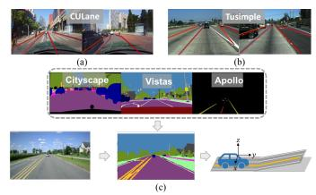
Fig 1. Comparison of labels among commonly used lane datasets and our training datasets. (a) (b) Examples with occluded/missing lane marks and lane labels; (c) Examples of our heterogeneous training datasets without labeling uncertainty, where the lane parameters are optimized based on scene labels without supervision.
