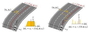
Fig. 6. Cost function for road fitting (left) and lane fitting (right)
