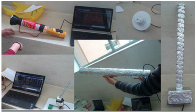
Fig. 4. Prototypes of WiFi antennas developed by students.
