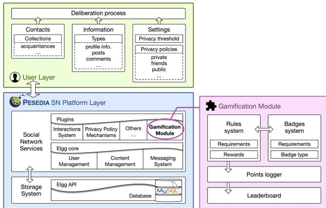
Fig. 1. Block diagram that represents the architecture of PESEDIA. Also represented is the relevant plugin for this work: the Gamification Module.
