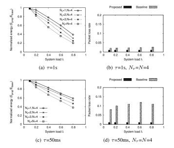
Fig. 6. Results for the relative energy consumption and the PLR of the proposed system versus the baseline system for different  $\lambda$  and *Scenario 1*.
