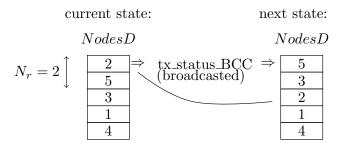
Fig. 5. Example that shows the ordered list *NodesD* at all nodes. We assume that node 2 will stop being a relay. The transmission of *STATUS\_BCC* that originates from node 2 will update *NodesD* at every node.
