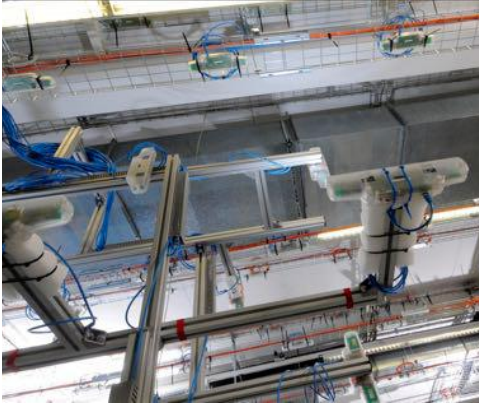
Fig. 7. Node deployment in the FIT IoT-LAB testbed.
