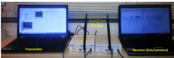
Fig. 7: Proposed USRP based experimental testbed.
