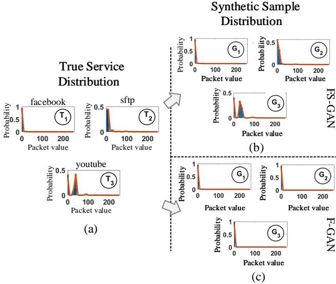
Fig. 1: Comparison between (a) the distribution of three service traffics  $T_1, T_2, T_3$  measured in packet value (converted decimal value of data packet) and (b) the synthesized traffic data produced by FS-GAN and (c) the synthesized traffic produced by F-GAN.
