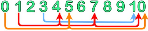
Fig. 3. Example of RRNS merge by using the Chinese Remainder Theorem.
