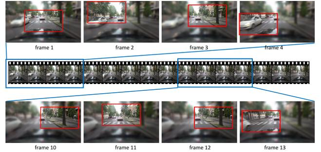
Fig. 3. A demonstration of the selective process mechanism. As the video plays sequentially, the sampler  $f_s(\theta_s)$  chooses a patch rather than processing the entire frame. At each time step, the sampler has observed several patches in previous steps. Based on these patches, the sampler determines where to locate to get more details. After the sampler obtains the patch to be processed, the sampler moves on to the next frame.
