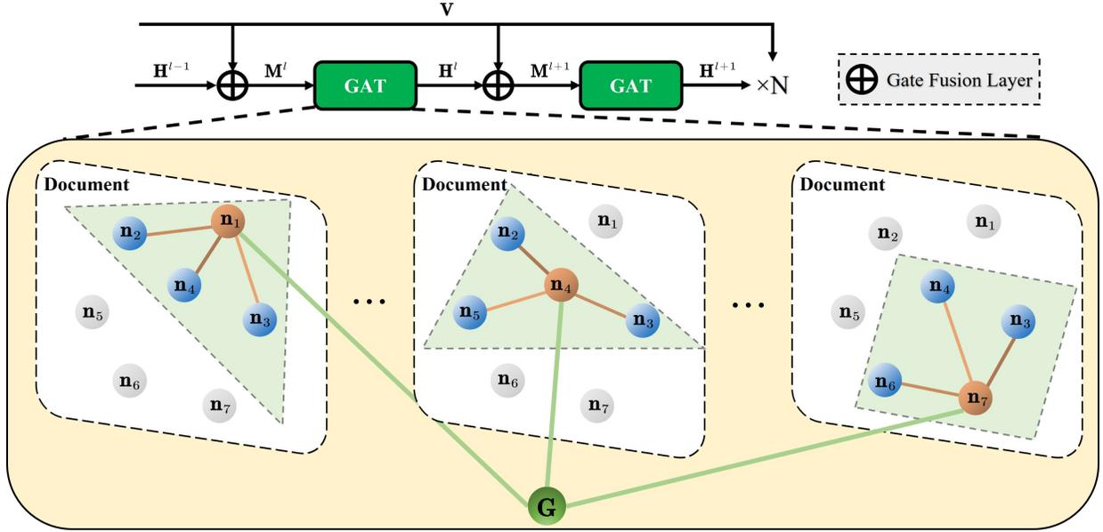
Fig. 5. An illustration of the graph attention layer. The  $\{\mathbf{n}_1 - \mathbf{n}_7\}$  represent different input nodes of the layer.  $\mathbf{G}$  is the global node, which assists each node to capture the global information of the document. Graph attention mechanism employed on  $\{\mathbf{n}_1, \mathbf{n}_4, \mathbf{n}_7\}$  is visualized.  $\{\mathbf{n}_1, \mathbf{n}_4, \mathbf{n}_7\}$  only attend to their neighborhood nodes and a global node  $\mathbf{G}$ .
