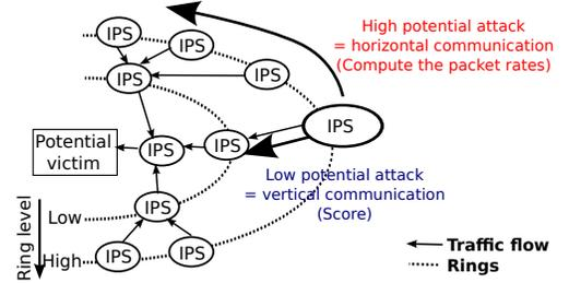
Fig. 2. Horizontal and Vertical communication in *FireCol*
