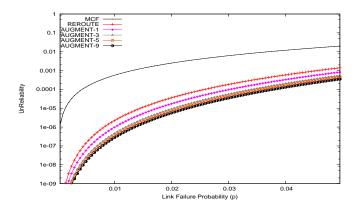
Fig. 12. Unreliability of different lightpath routings.
