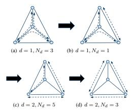
Fig. 4. Improving reliability via lightpath rerouting. The physical topology is in solid lines, and the lightpath routing of the logical topology is in dashed lines. The MCLC value and the number of MCLCs in the lightpath routings are denoted by d and  $N_d$ .
