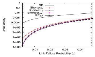
Fig. 8. Lightpath rerouting: performance of approximation algorithm.
