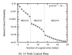
Fig. 10. Impact on reliability by augmenting logical rings.
