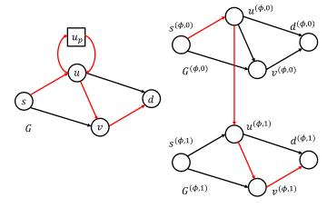
Fig. 2. The left figure is the original graph  $\mathcal{G}$ , where u is the only computation node for the single function in  $\phi$ . A dummy node  $u_p$  and connections to u are added to illustrate the availability of service function processing at node u. The right figure is the layered graph  $\mathcal{G}^{(\phi)}$ .
