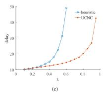
Fig. 5. Average packet delay performance: (a) UCNC v.s. backpressure-based algorithm; (b) UCNC v.s. nearest-to-destination function placement heuristic; (c) UCNC v.s. nearest-to-source function placement heuristic.
