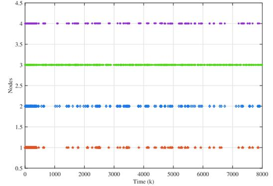
Fig. 8. Updating instants of the controller input under the DDET mechanism.
