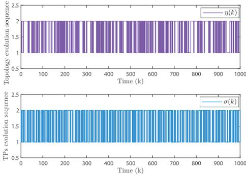
Fig. 3. Possible evolution sequence of the topology switching  $\eta(k)$  and TPs switching  $\sigma(k)$ .
