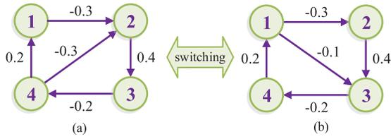
Fig. 2. Switching topologies  $\mathcal{G}^1$  and  $\mathcal{G}^2$ . (a) Signed graph  $\mathcal{G}^1$ . (b) Signed graph  $\mathcal{G}^2$ .
