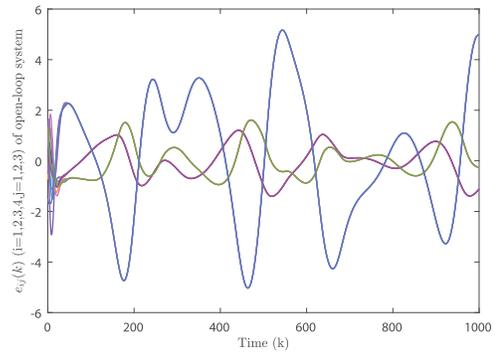
Fig. 4. Bipartite synchronization errors of the open-loop system.
