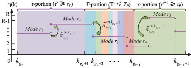
Fig. 1. Possible switching sequence of  $\{\eta(k), k \in [k_{g_v}, k_{g_{v+1}+1}]\}$  under PDT switching regularity.
