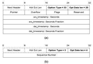
Fig. 1. Unidirectional (a) packet delay and (b) packet loss IPv6 destination options
