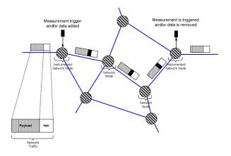
Fig. 2. In-line Measurement Operation
