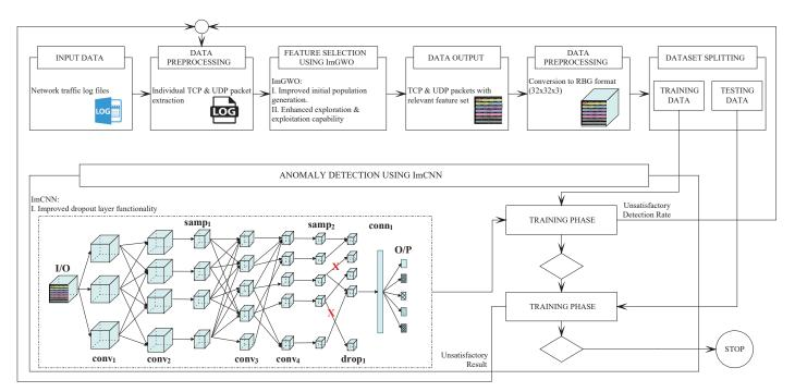
Fig. 1: Proposed hybrid model using ImGWO and ImCNN for network anomaly detection in cloud setup.
