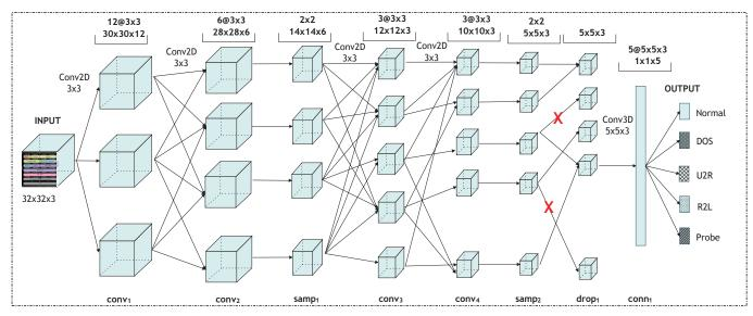
Fig. 2: The architecture of the ImCNN used for network anomaly detection for streaming data in cloud setup.
