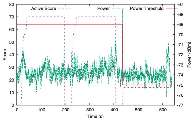
Fig. 9: Active IM score of the SCATTER system in a Passive Incumbent Environment of a Solo game.
