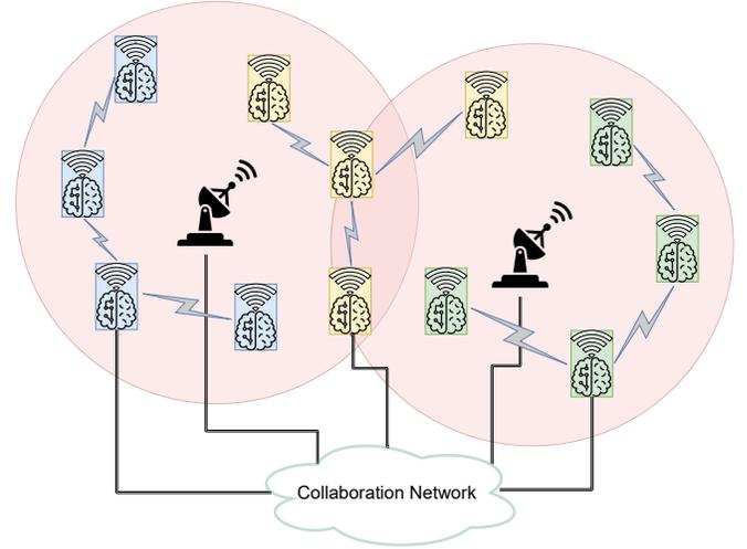
Fig. 1: Network topology with three networks (blue, yellow and green) and two incumbents (black). Each network has one gateway which is connected to a wired backbone and has the ability to communicate with other gateways and collaboration-enabled incumbents.
