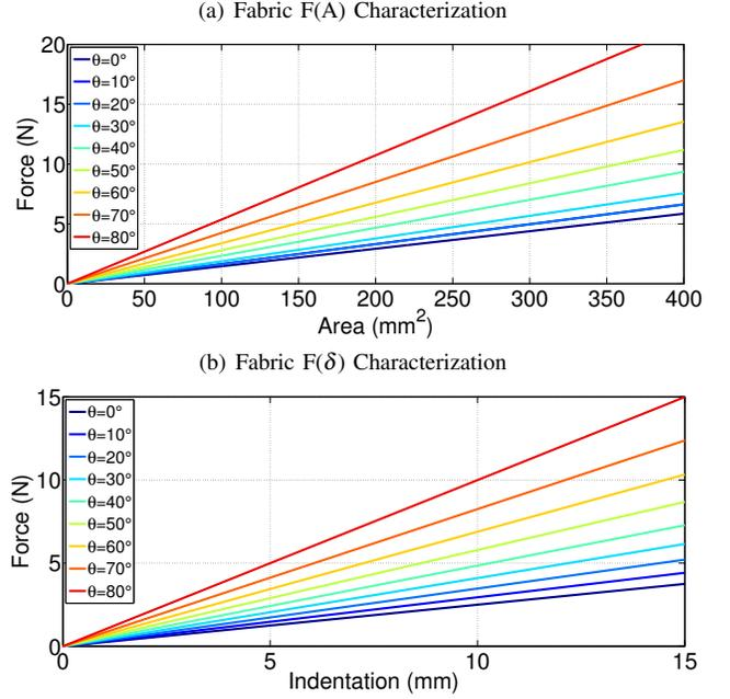
**Fig. 5:** (a):  $F(A)$  curves of FYD-2 at different motor positions; (b):  $F(\delta)$  curves of FYD-2 at different motor positions.
