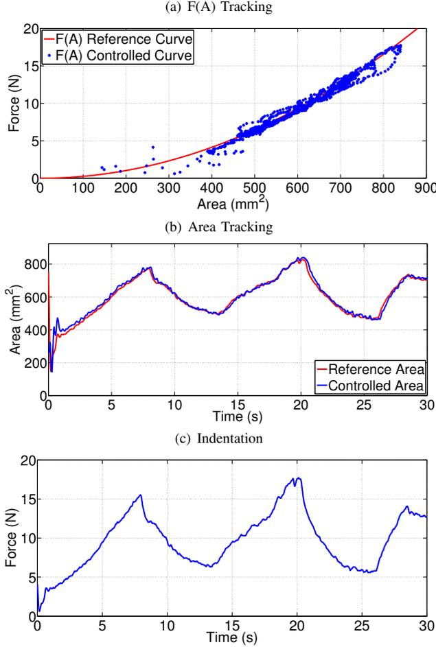
**Fig. 9:** In the first plot (a) we show the reference  $F(A)$  curve (in red), while the pairs (measured controlled area, measured force) are represented as blue dots. In the second plot (b) we report the contact area control (blue line) vs. contact area reference (red line). In the third plot (c) the measured force is reported. These plots refer to the silicone specimen SS1.
