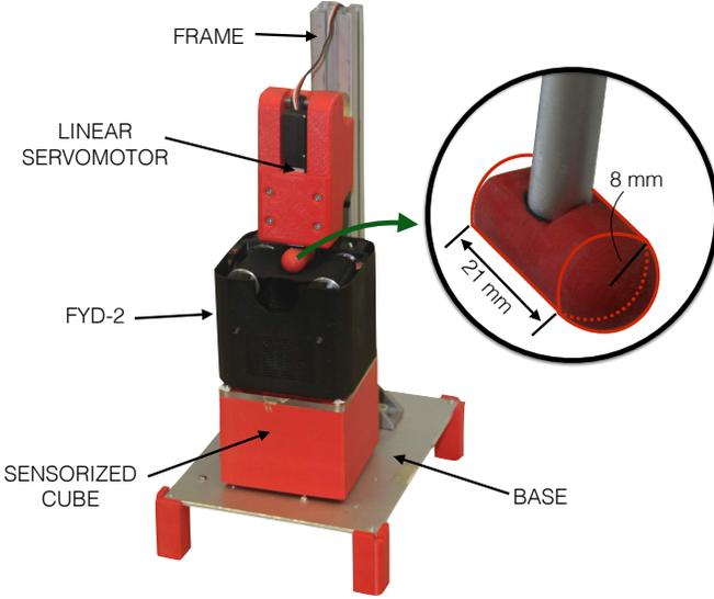
**Fig. 4:** The indenter used to characterize the FYD-2 and the silicone specimens. In the sensorized cube we placed a webcam and a load cell.
