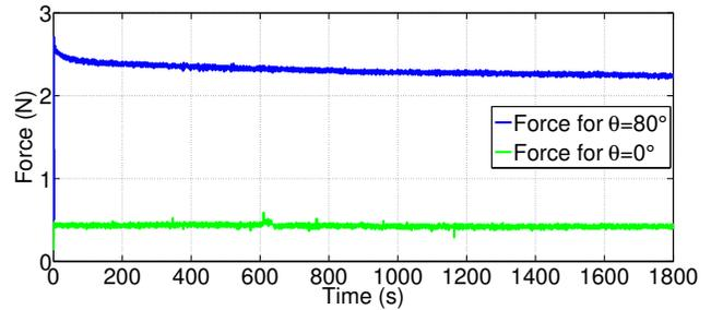
**Fig. 6:** Stress-Relaxation test of the fabric used in the FYD-2 for  $\theta = 0^\circ$  and for  $\theta = 80^\circ$ .
