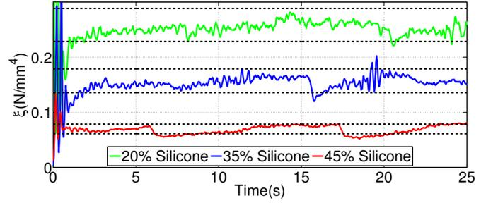
**Fig. 10:** Control of  $\xi_r$  for the three silicone specimens, which were used also for the experiments with humans reported in Section 4. The dashed black lines define the 5% error bounds.
