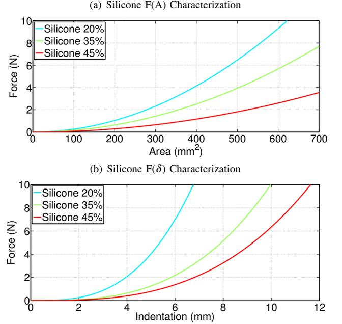
**Fig. 11:** The  $F(A)$  characteristics of the three silicone specimens used for the experiments with humans (see also Section 4). Silicone 20% corresponds to SS1, while Silicone 35% and Silicone 45% can be referred to as SS2 and SS3, respectively.
