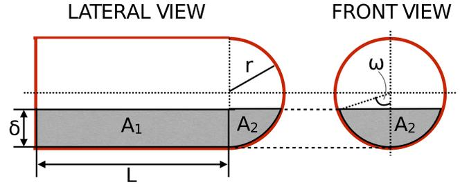
Fig. 7: The indenter: sketch and main geometric features ( $r = 8$  mm,  $L = 20$  mm).  $\delta$  indicates the indentation produced by the indenter on the fabric surface. The shadow parts belong to the contact area of the indenter with the fabric.
