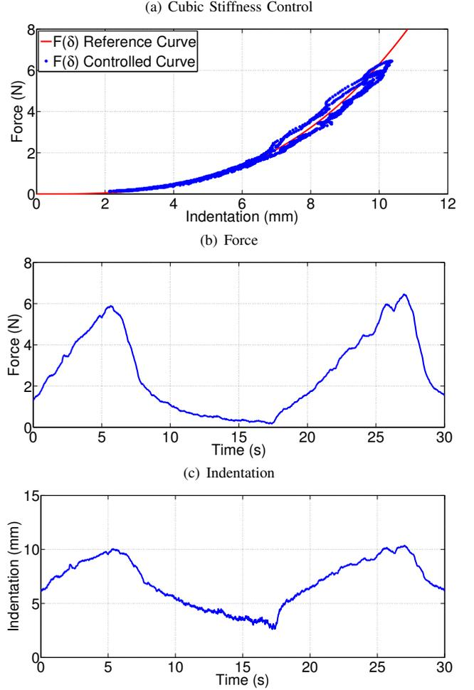
**Fig. 13:** Tracking of force-indentation characteristic of SS3 and time-evolution of measured force and estimated indentation, respectively.
