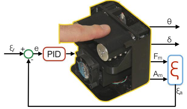
Fig. 8: Control scheme for  $F(A)$  tracking.
