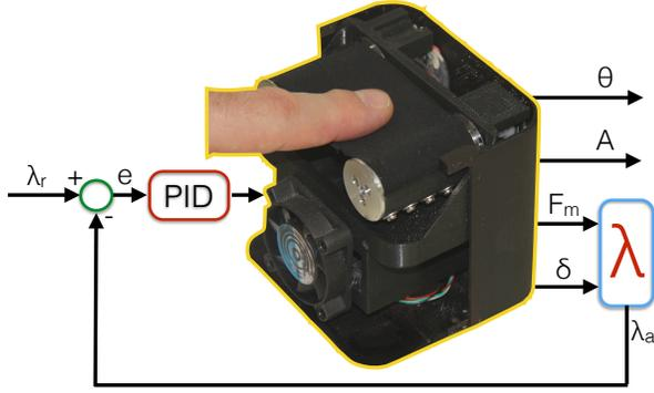
**Fig. 12:** Control scheme used for force - indentation tracking experiments.
