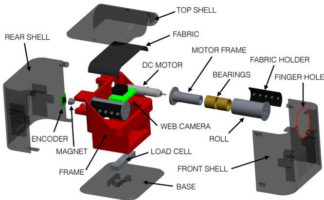
**Fig. 2:** Exploded drawing of the FYD-2.
