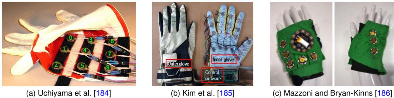
Fig. 5. Three representative wearable haptic devices providing vibrotactile stimuli to the hand.
