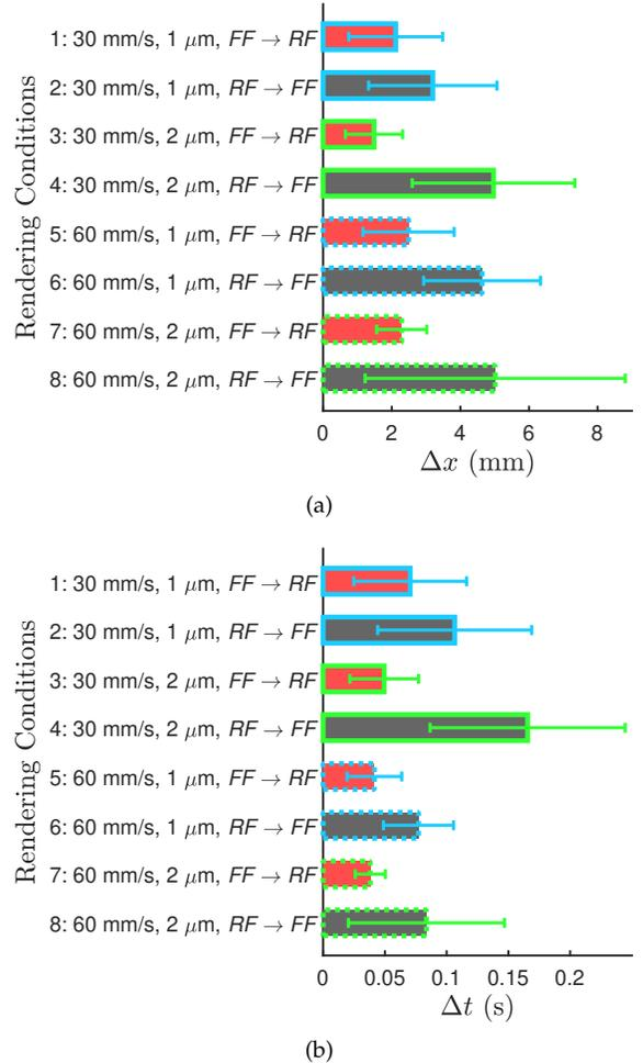
Fig. 4: Thresholds to discriminate two consecutive virtual edges in EXP-1 (mean values and standard deviations); a) spatial threshold and b) temporal threshold. Red and gray bars are for  $FF \rightarrow RF$  and  $RF \rightarrow FF$ , solid and dotted bars are for  $f_v$  of 30 and 60 mm/s, blue and green bars are for  $V_{amp}$  of 1 and 2  $\mu m$ , respectively.
