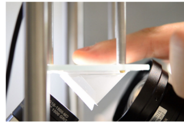
Fig. 1. A soft finger's contact area develops in various ways depending on its material properties and how it is pressed into the surface.
