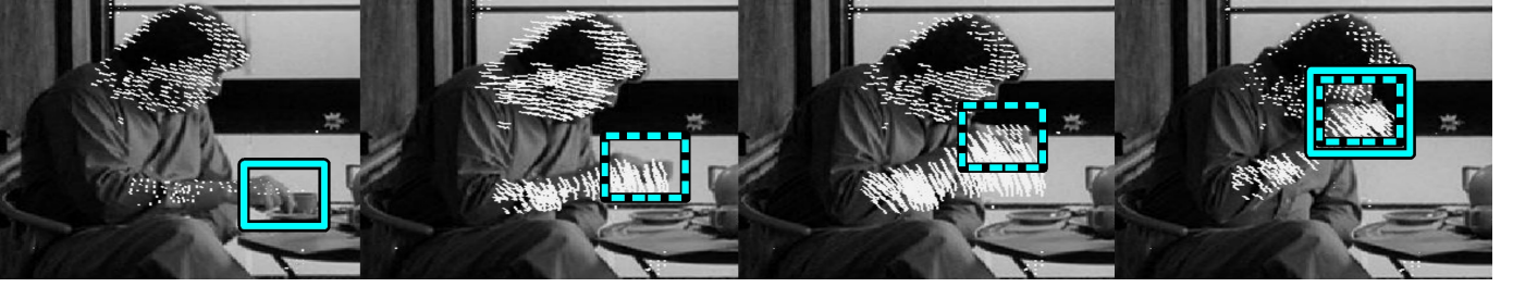
Fig. 4. The DPT-MS tracker at test time. In the first frame (left) the cup is automatically detected by an object detector. In the subsequent frames no detections are found on the cup. DPT-MS produces an object track (dashed window) by propagating the detection from the first frame according to point tracks (white segments). In the last frame (right) the cup is again detected. DPT-MS adds this detection to the track and uses it to update the confidence score, but not the location of the track.
