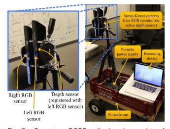
Fig. 7. Our stereo-RGBD collection rig consists of two side-by-side Microsoft Kinects. The rig is mobile through the use of an uninterruptible power supply, laptop, and rolling mount.
