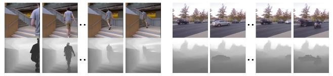
Fig. 1. Our technique takes a video sequence (*top row*) and automatically estimates per-pixel depth (*bottom row*). Our method does not require any cues from motion parallax or static scene elements; these videos were captured using a stationary camera with multiple moving objects.
