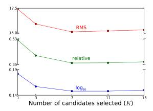
Fig. 15. Effect of the number of chosen candidates (K). Errors are reported on the Make3D dataset with varying values of K. For this dataset, K=7 is optimal, but increasing K beyond 7 does not significantly degrade results.
