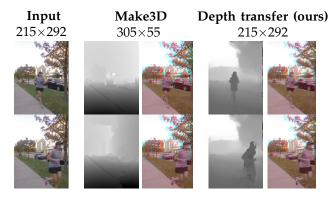
Fig. 14. Comparison between our technique and the publicly available version of Make3D (http://make3d. cs.cornell.edu/code.html). Make3D depth inference is trained to produce depths of resolution  $55\times305$  (bilinearly resampled for visualization), and we show results of our algorithm at the input native resolution. The anaglyph images are produced using the technique in Sec 7. Depths displayed at same scale.
