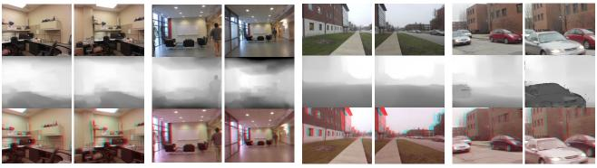
Fig. 11. Results obtained on four different sequences captured with a rotating camera and/or variable focal length. We show the input frames (*top*), inferred depth (*middle*) and inferred 3D anaglyph (*bottom*). Notice that the sequences are time-coherent and that moving objects are not ignored.
