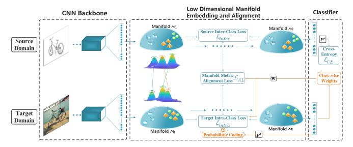
Fig. 2. Overview of the proposed multilayer Riemannian manifolds embedding and alignment network. A CNN-based feature extractor is adopted to learn the common representations of both domains. The discriminative information are transferred via the Riemannian manifold layers, where fully connected layers are equipped with the proposed proposed soft discriminant criterion and manifold metric domain alignment. Best viewed in color.
