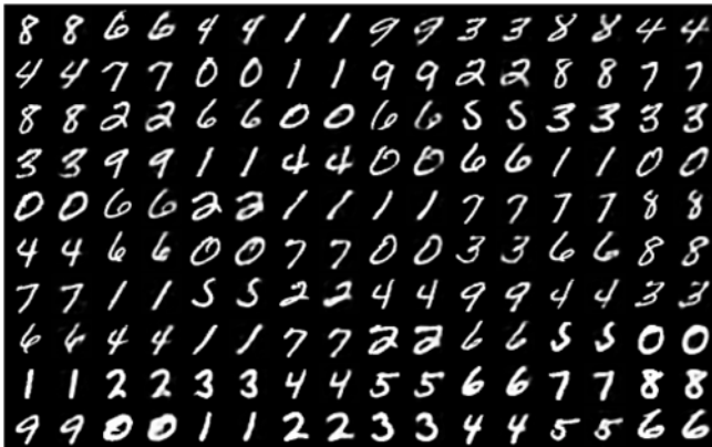
Fig. 8. Illustration of the reconstructed images from spiking autoencoder ( N_s = 32 ) on the MNIST dataset. For each pair of digits, the left side is the original image and the right side is the reconstruction by SNN.
