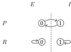
Fig. 4: A simple TA with two states. In this figure, “P”, “R”, “I”, and “E” means “penalty”, “reward”, “include” and “exclude” respectively.
