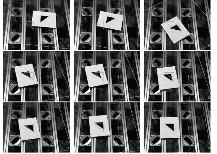
Fig. 6. Underactuated distributed manipulation movie snapshots. The goal is to align the black triangle affixed to the plexiglass with the superimposed triangle.
