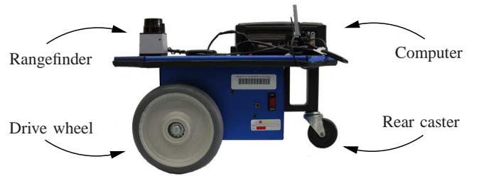
Fig. 6. Erratic mobile robot with URG-04LX laser rangefinder.
