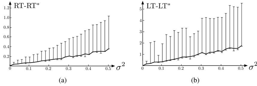
Fig. 9. For the roadmap in Fig. 7, 100 team trajectories have been generated with Algorithm 5 for each value of  $\sigma^2$ . The average refresh time and the average latency are plotted as continuous lines in Fig. 9(a) and Fig. 9(b) respectively. The bars indicate the minimum and the maximum value of the refresh time and the latency, respectively. Notice that the average team trajectory performance degrade gracefully with the noise variance.
