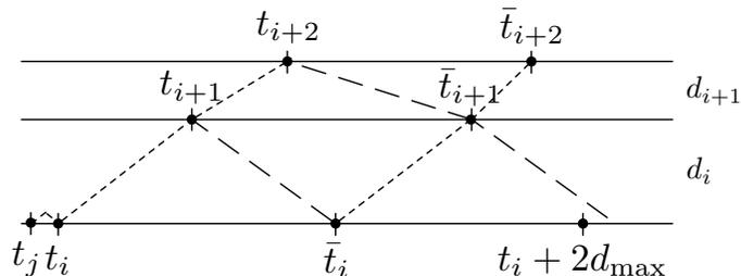
Fig. 5. As stated in Lemma IV.3, at most one communication sequence is possible within each period of length  $2d_{\max}$ . Here  $d_i + d_{i+1} > d_{\max}$ .
