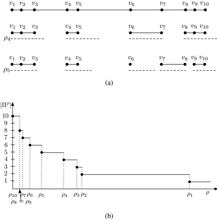
Fig. 3. In 3(a) the left-induced partition of length  $\rho_4$  and  $\rho_5$ , with  $\rho_5 < \rho_4$ , for the chain roadmap with vertices  $\{v_1, \dots, v_{10}\}$ . The cardinalities are  $|\Pi^{\rho_4}| = 4$  and  $|\Pi^{\rho_5}| = 5$ , respectively. In 3(b) the cardinality  $|\Pi^\rho|$  is plotted as a function of the length  $\rho$ . Notice that, because  $v_2 - v_1 = v_{10} - v_9$ , the function  $|\Pi^\rho|$  does not assume the value 9.
