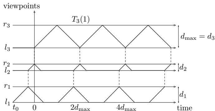
Fig. 4. A team trajectory with minimum up-latency generated with the procedure in Trajectory 3. Notice that each robot  $i$  communicates with the neighboring robot  $i+1$  as soon as  $x_i(t) = r_i$ . A team trajectory with minimum down-latency is obtained by shifting in time the trajectory of robot 1, in a way that robot 2 communicates with robot 1 as soon as  $x_2(t) = l_2$ .
