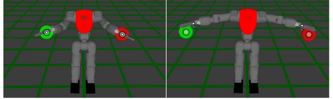
Fig. 12: Illustration of the waist joint prioritization problem. **Left:** Both targets are within the reachable workspace of both arms, so the robot can successfully reach the centers of the spheres with the palm of its hands. **Right:** References become simultaneously unreachable, so the robot cannot reach any of the two. The small circles depict the tool center point of each arm, while the large circles represent the centers of the references.
