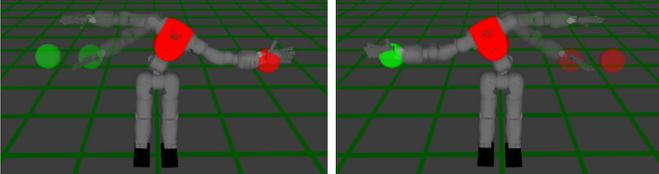
Fig. 14: Movement synthesis using the learned left and right arm priority models. **Left:** The left reference is always tracked, while the right reference is only tracked when reachable. **Right:** The right reference is prioritized.
