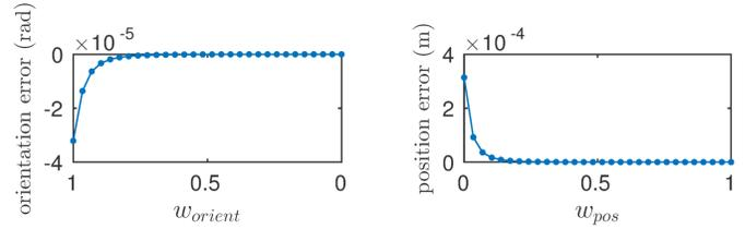
Fig. 11: Performance of the robot in tracking position and orientation references with varying weights when both tasks can be achieved
