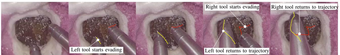
Fig. 15. Snapshots of the tool evasion in the third automatic tracing experiment, in which both robots moved. The left tool uses the dynamic knowledge of the right tool to initiate the evasive maneuvers before getting close to it.
