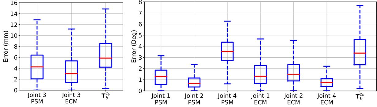
Fig. 6: Box plots of the tracked joint angle errors, whose preceding kinematic links are never in the camera frame, and the base of camera arm to base of robotic tool transform,  $\mathbf{T}_b^{c_b}$ , error when explicitly estimating all unknowns in the simulated da Vinci scene. Errors up to 14mm and 7 degrees highlight the inability to estimate these unknown values explicitly due to the parameters being non-identifiable as shown in Claim 1.
