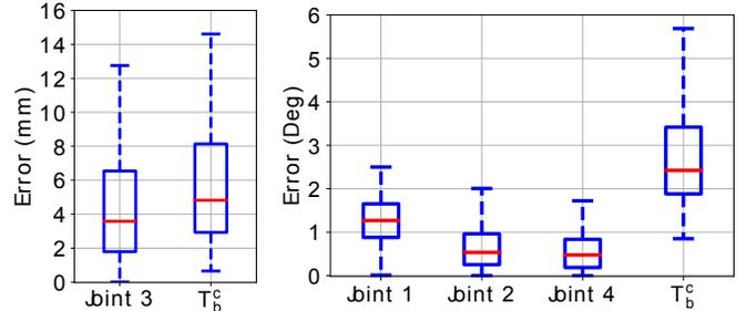
Fig. 5: Distribution of first 4 joint angle errors, whose preceding kinematic links are never in the camera frame, and the stationary camera to base transform,  $\mathbf{T}_b^c$ , error when explicitly estimating them in the simulated da Vinci scene. Errors up to 14mm and 5 degrees highlight the inability to estimate these unknown values explicitly due to the parameters being non-identifiable as shown in Claim 1.
