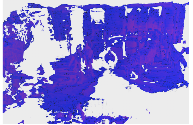
Fig. 9: Single-robot reconstruction of the Cow and Lady dataset [37]. Red hues indicate lower TSDF variance.
