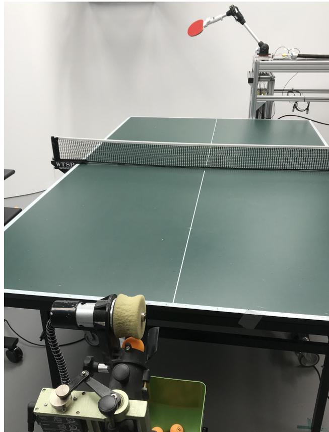
Fig. 1: Our setup consists of a four DoF robot arm actuated by pneumatic muscles and a ballgun that launches balls towards the robot arm. The robot successfully learns to return the ball to a desired landing point on the table. The Cartesian positions of the ball are measured by a color-based camera detection system.
