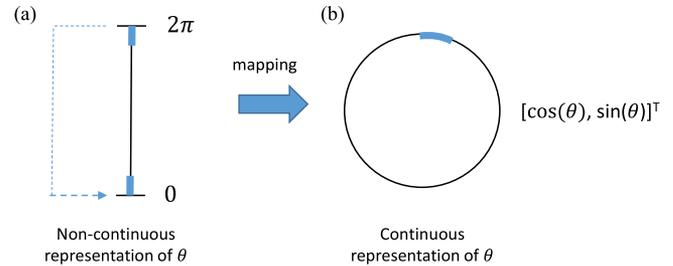
Fig. 8. Instead of directly estimating the angle of the bending plane, the proposed MLP divides it into two outputs, i.e., the sine and cosine of the angle of the bending plane. This approach transforms the discontinuous rotation representation (left) into a continuous representation (right), thus facilitating the fitting of the neural network.
