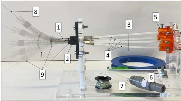
Fig. 1. Two-DOF fluidics-driven catheter system for data acquisition and algorithm validation: 1—distal catheter segment; 2—catheter segment clamp; 3—FBG fiber; 4—PAMs; 5—PAM clamp; 6—adjustable back plate; 7—EM sensor connector; 8—protective Nitinol tube; 9—heat shrink.
