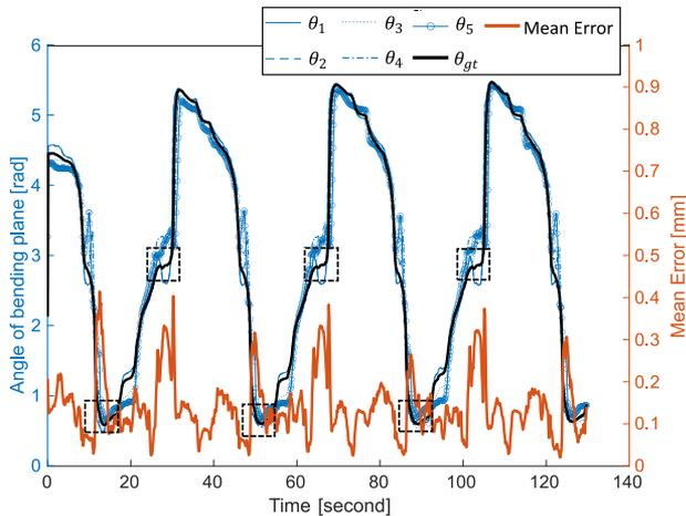
Fig. 13. Estimated angles of the bending plane of each grating (blue), ground truth angle of the bending plane (black), and mean error (orange) of Lissajous (1) experiment are plotted over the time. The transition regions where there are increases in mean error are marked with dashed square.
