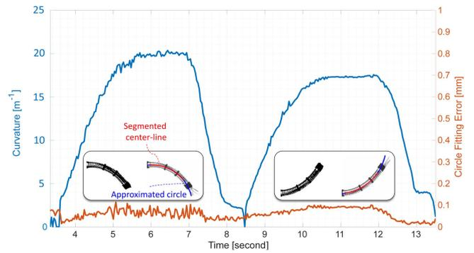
Fig. 3. Result of constant curvature verification experiment. The threshold images and the fitted circles can be seen in the inserts. The estimated curvature and errors of circle approximations are shown in blue and red, respectively.
