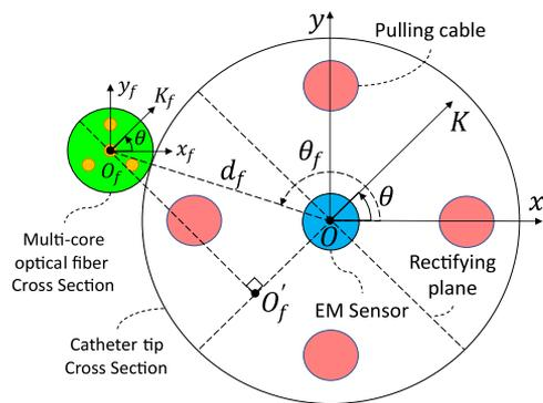
Fig. 6. Cross-sectional view of the catheter tip and the multicore FBG fiber, where  $\theta$  is the angle of the bending plane with respect to the  $x$ -axis,  $d_f$  is the distance between the center of the catheter and the fiber's central axis, and  $\theta_f$  is the angle between the  $x$ -axis and the center of the fiber  $O_f$ .
