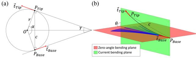
Fig. 4. Example of curvature and angle of the bending plane calculation along explanation of Section III-B. (a) Curvature calculation. (b)  $\theta$  is the angle between the zero-angle bending plane and the current bending plane.
