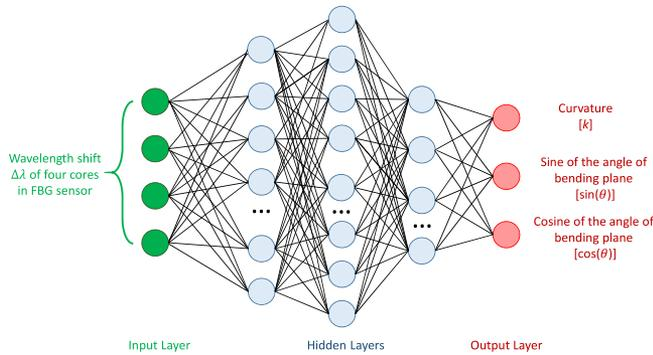
Fig. 7. MLP for estimating curvature and angle of bending plane. The four wavelength shifts  $\Delta\lambda$  from the four-core FBG fibers are entered into the input layer of the proposed MLP. The output layer has three neurons. One neuron predicts the curvature, while the other two predict the sine and the cosine of the angle of the bending plane. Five of these MLPs are established for the five gratings that are distributed over the entire length of the catheter segment.
