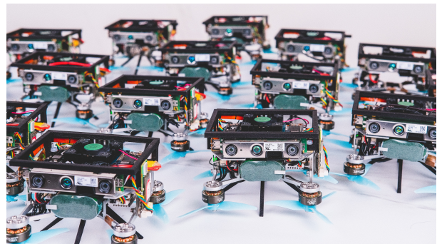
Fig. 12. Illustration of palm-sized swarm aerial robots.
