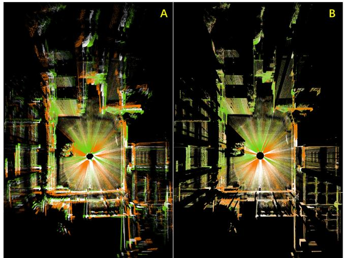
Fig. 14. The point cloud of MID-100 lidar in Scene-1 reconstructed before (A) and after (B) extrinsic optimization. The base lidar ( $L_1$ ) point cloud is colored in white and the two lidars to be calibrated ( $L_0$ ,  $L_2$ ) are colored in orange and green, respectively.
