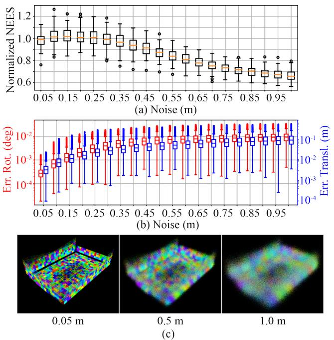
Fig. 7. (a) The normalized NEES averaged over 100 Monte Carlo runs at different point noise levels. The NEES is normalized by the pose dimension (i.e., 600) for better visualization. (b) The rotation (red) and translation (blue) errors at different point noise levels. (c) The point cloud map with ground-true poses at noise levels  $\sigma_p = 0.05\text{m}$ ,  $0.5\text{m}$  and  $1\text{m}$ , respectively.
