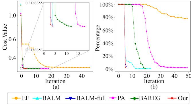
Fig. 8. Convergence of different methods in BA optimization. (a) Cost convergence in one repeat experiment of the nominal settings  $M_f = 40$ ,  $M_p = 40$  and  $N = 40$  in one repeat experiment. (b) Iteration steps experienced by each method in all repeat experiments (i.e., 10) of all scenes (i.e., 13). The y-axis value represents how many experiments out of the total (130) has experienced the iteration number indicated on the x-axis.
