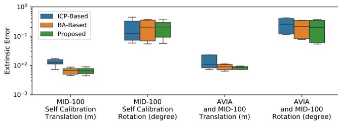
Fig. 13. Extrinsic calibration results of the ICP-based [22], BALM-based [69] and our proposed method in two experiment setups (with small or without FoV overlap).
