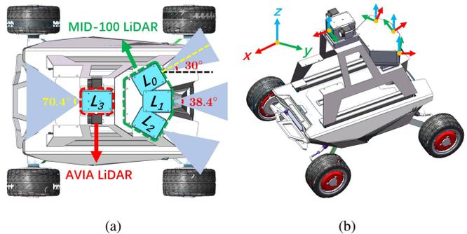
Fig. 12. The customized multi-sensor vehicle platform in [69]. The MID-100 lidar consists of three lidars:  $L_0$ ,  $L_1$  and  $L_2$ , with FoV overlap between adjacent lidars  $8.4^\circ$ . The AVIA lidar is denoted as  $L_3$ . (a) The FoV coverage of each lidar sensor. (b) Each lidar sensor’s orientation denoted in the right-handed coordinate system.
