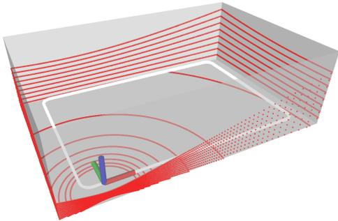
Fig. 5. Simulation setup: A 16-channel lidar moves along a rectangular trajectory in a cuboid semi-closed space. The white line is the trajectory and the red lines are the laser points.
