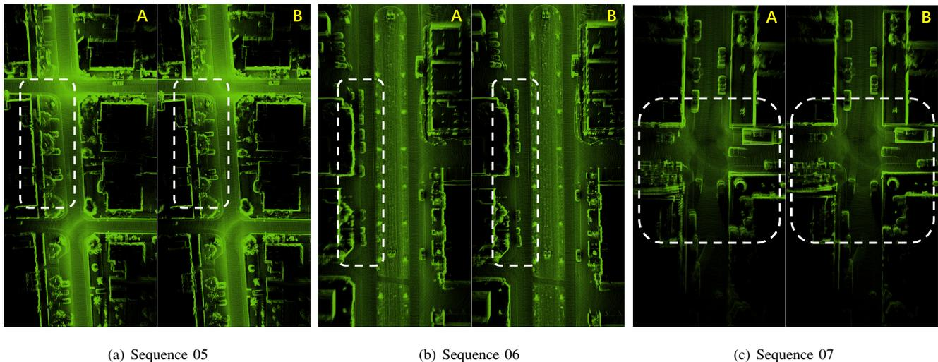
Fig. 15. Comparison of odometry accuracy on KITTI dataset [71]. The left image (A) of each subplot depicts the point cloud reconstructed by MULS [70] which is used as our initial value. The right image (B) of each subplot is the point cloud optimized by our proposed global BA method. The white dashed rectangle emphasized the difference (zoomed view is recommended).
