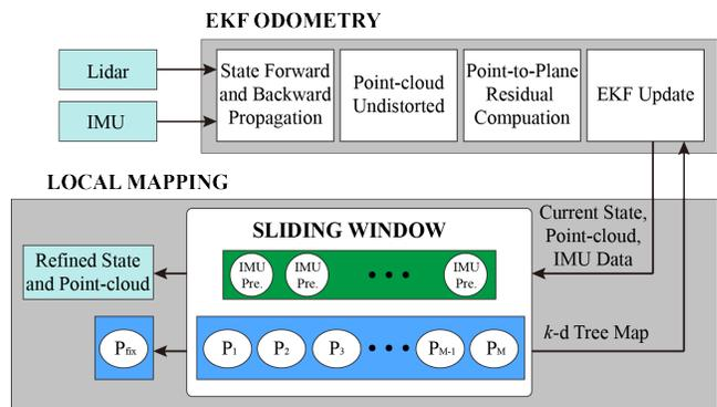
Fig. 11. Overview of the LIO system with BA and IMU preintegration
