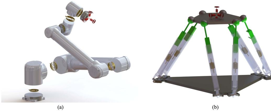
Fig. 1. Compliant robotic systems. The yellow virtual springs characterize the flexibility of the system in joint space, and the red virtual springs characterize the flexibility of the system in Cartesian space as it interacts with the environment. (a) The serial manipulator with virtual springs. (b) The parallel manipulator with virtual springs.
