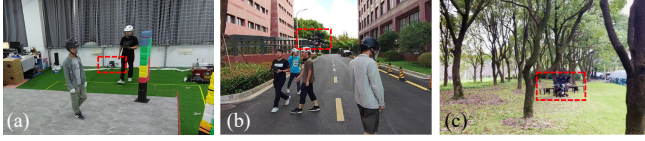
Fig. 15. The testing scenarios for obstacle avoidance. (a) and (b) are dynamic environments. (c) is a static environment. Red rectangles outline the quadrotor.
