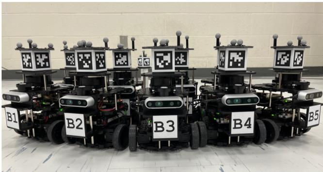
Fig. 9: Image of a Turtlebot3 Burger used in the real robot experiment. It is fitted with AprilTag-labelled cubes, an Intel-Realsense D435i camera and Vicon markers. Vicon markers are only used to obtain the ground-truth trajectories, used for the evaluation. The depth image, laser scanner and IMU are not used in any of the experiments.
