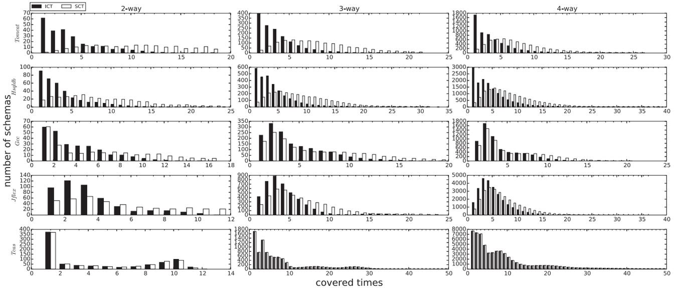
Fig. 3. The redundancy of test cases.
