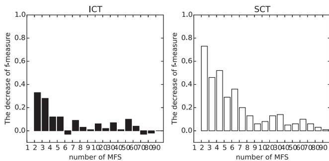
Fig. 10. The decrease of F-measure (multiple MFS in one test case) for various numbers of MFS.
