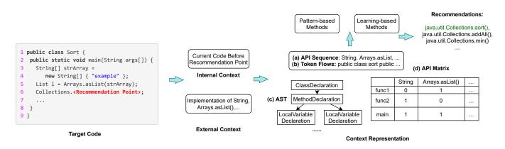
Fig. 2. The typical code-based API recommendation framework.
