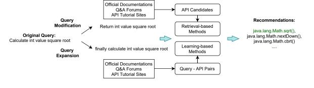
Fig. 1. The typical query-based API recommendation framework.
