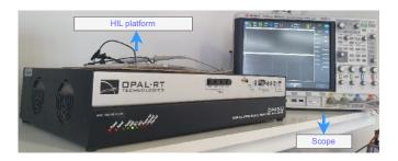
Fig. 11. OPAL-RT platform for HIL validation
