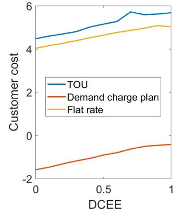
Fig. 8. Customer cost under varying DC meter estimation error.
