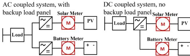
Fig. 1. Future Meter Placement Demonstration. The highlighted red meters are fictitious positions for DC meters.
