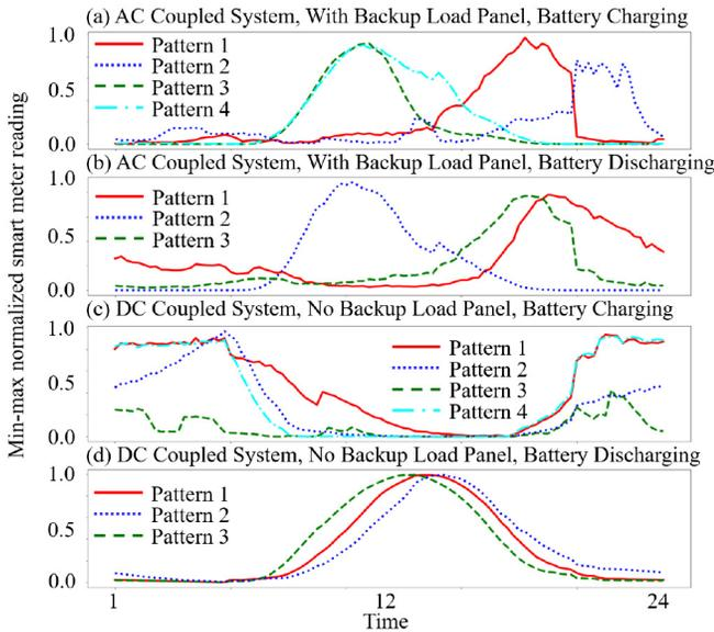
Fig. 3. Raw data and clustered battery meter data patterns. The x-axis is the hours during a whole day. The y-axis is the value of the raw data after min-max normalization.
