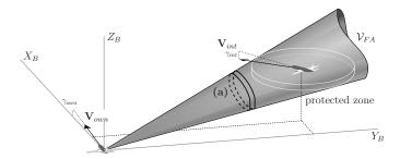
Fig. 4. The 3-D forbidden area  $\mathcal{V}_{FA}$  consists of a conical area that is aligned with the edges of the intruder protected zone, as seen from the ownship, and has its apex situated at the center of ownship. Cross-section (a) shows how the thickness of the protected zone changes the shape of the forbidden area from what would otherwise be a pure slanted cone, to a combination of two slanted cones, connected by a straight section.
