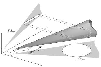
Fig. 6. Translated 3-D forbidden area and horizontal and vertical projections.  $FA_{hor}$  is the horizontal projection of the 3-D forbidden area, and presents constraints for ownship track and horizontal velocity.  $FA_{ver}$  is the vertical projection of the same area, and presents constraints for vertical motion.
