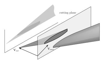
Fig. 8. The vertical reduced constraint area is given by the intersection of the 3-D constraint area, and a vertical cutting plane, aligned with the ownship track. The vertical reduced area illustrates exact constraints on vertical maneuvering, also for conflicts with non-zero cross-track distances and velocities.
