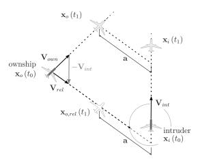
Fig. 3. Relation between ownship motion relative to the intruder, and the absolute motion of ownship and intruder. Ownship and intruder are shown at time  $t_0$  and  $t_1$ .  $\mathbf{x}_{o,rel}$  shows how ownship has moved *relative* to the intruder. Line  $\mathbf{a}$  shows that the change in orientation between ownship and intruder along the relative path is equal to the change along the absolute paths.
