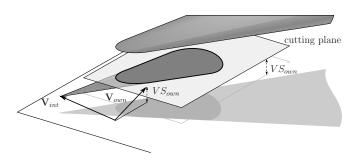
Fig. 7. The horizontal reduced constraint area is given by the intersection of the 3-D constraint area, and a horizontal cutting plane, offset vertically by the ownship vertical speed. The horizontal reduced area illustrates exact constraints on horizontal maneuvering, also for conflicts with non-zero relative vertical distances and velocities.
