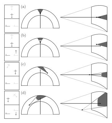
Fig. 12. Example scenarios. An overview of each scenario is given on the left. The black aircraft symbols represent ownship, the gray symbols represent the intruder. (a) Ownship is behind and overtaking the intruder, both are flying level, at equal altitude. (b) Intruder is climbing. (c) Both are flying level, but the intruder is to the left of ownship, crossing to the right. (d) Intruder is to the right of ownship, crossing to the left, descending from a higher altitude.
