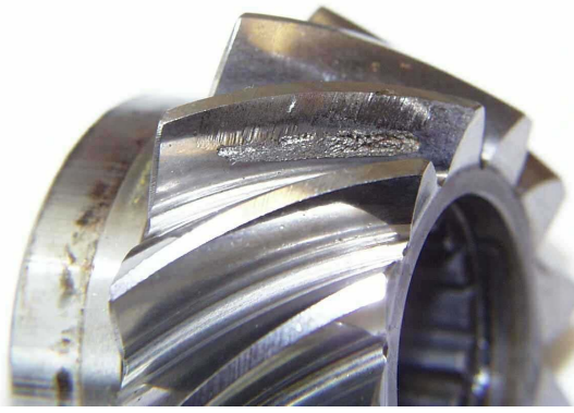
Fig. 6. Damaged spiral bevel gear.
