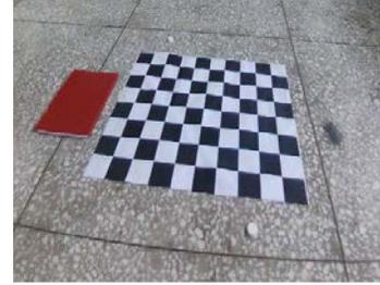
Fig. 12. Distorted checkerboard calibration pattern.
