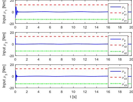
Fig. 3. Control input  $\mu$  under model-based control (23).
